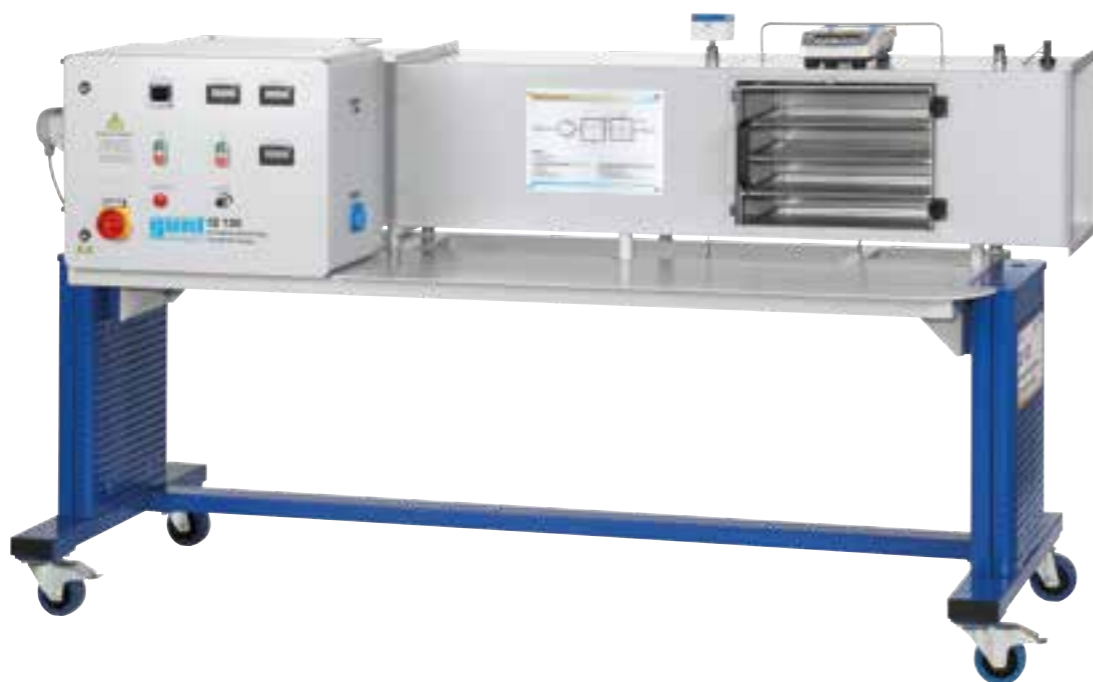
CE 130 Convection drying Drying curves for granular solids
