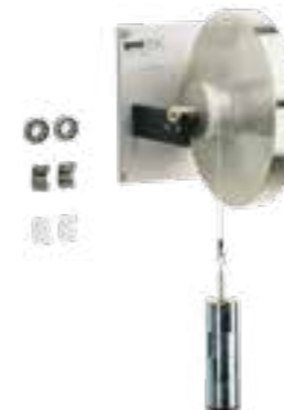
TM 282 Friction in journal bearings Learning the fundamentals of hydrodynamic lubrication by experimentation
