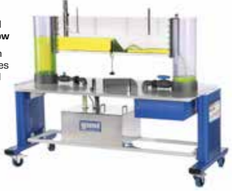
HM 111 Pipe networks Pressure losses at various piping elements and pipe networks; parallel and series connection of pipe sections
