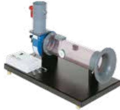
HM 240 Principles of air flow Recording the fan characteristic
