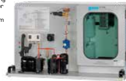
ET 352.01 Solar heat for refrigeration Solar thermal operation of a vapour jet compressor
