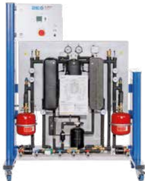
HL 320.01 Heat pump Heat pump for operation with different sources, operating the heating controller via web browser
