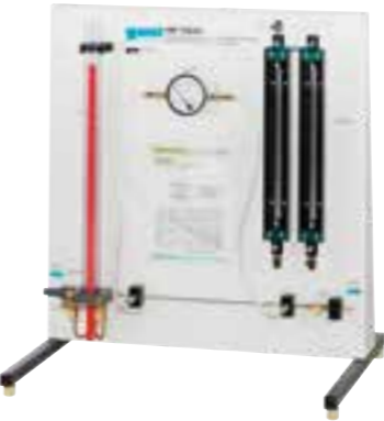
HM 150.01 Pipe friction for laminar/turbulent flow Determining the critical Reynolds number Recommended for water supply: HM 150 Base module for experiments in fluid mechanics
