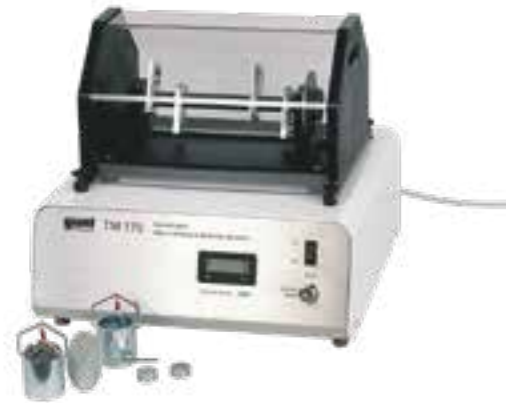
TM 170 Balancing apparatus Demonstration of the fundamentals of static and dynamic balancing
