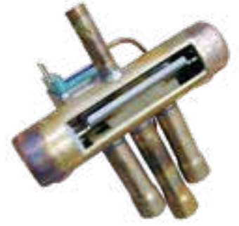
ET 499.25 Cutaway model: 4-way reversing valve
