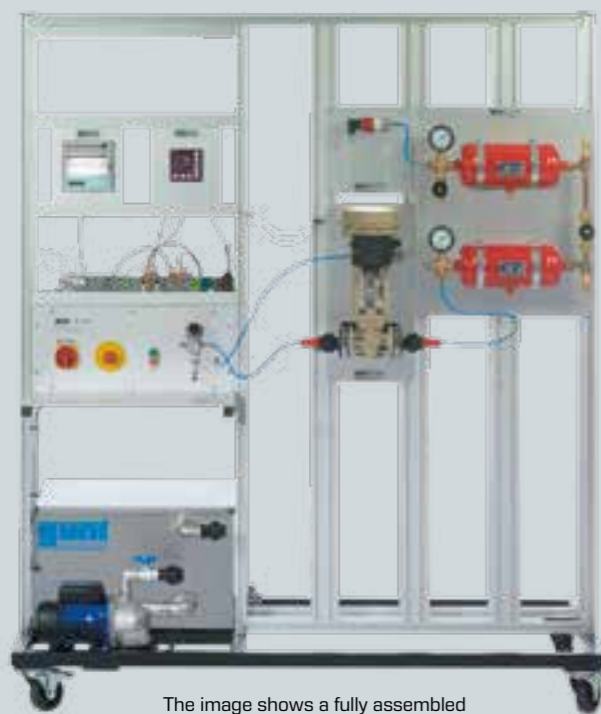
The image shows a fully assembled pressure control system after planning and execution of the piping and wiring.
