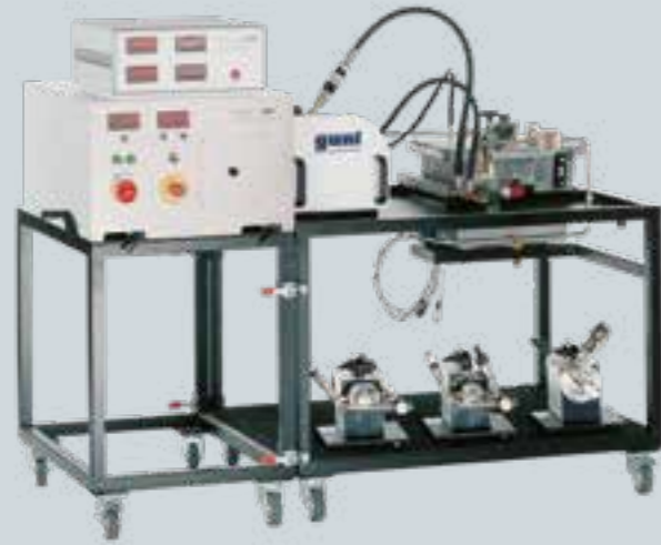
Trainer for positive displacement pumps with supply unit HM 365.20, screw pump HM 365.21 and drive unit HM 365
