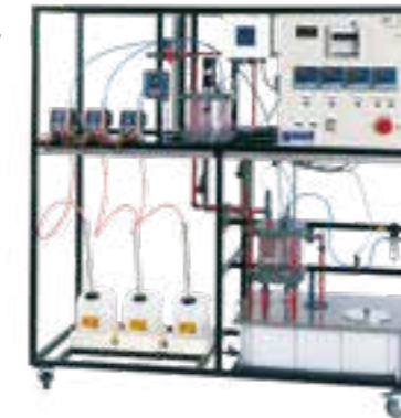
RT 586 Control of water quality Control of pH value, redox potential, oxygen concentration and electrical conductivity
