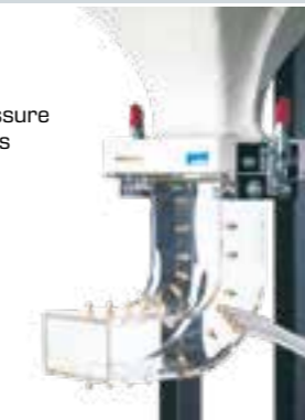
HM 225.07 Free jet Investigation of flow from nozzles
