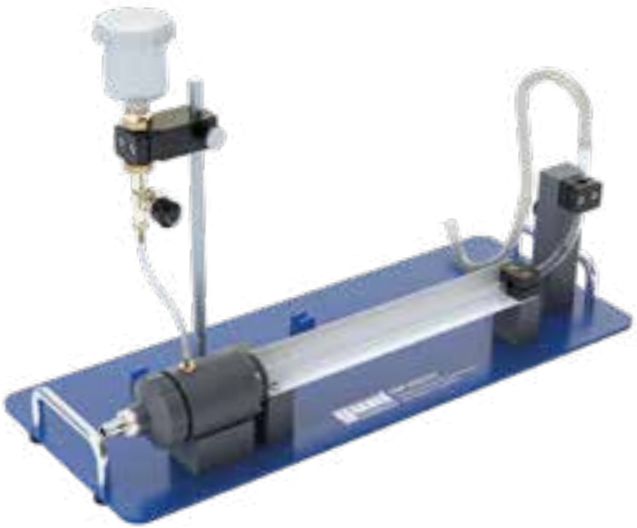
HM 250.08 Losses in pipe elements Influence of flow velocity on pressure loss, didactically successive pipe sections
