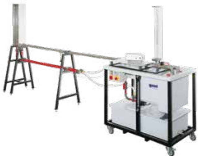
HM 156 Water hammer and surge chamber Investigation of formation, effect and function
