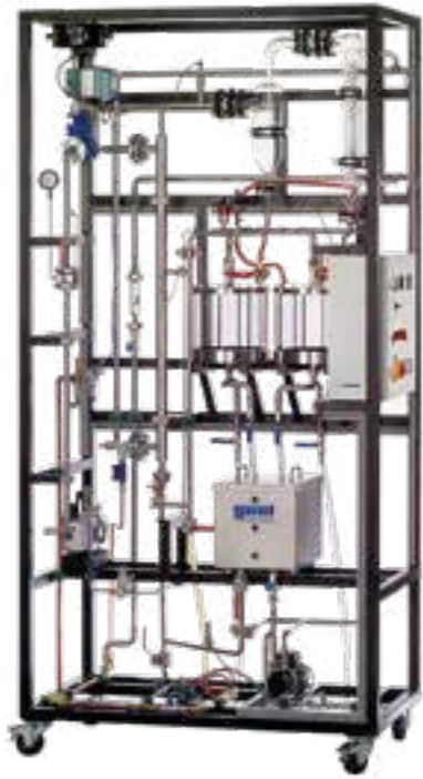
CE 130 Convection drying Drying curves for granular solids
