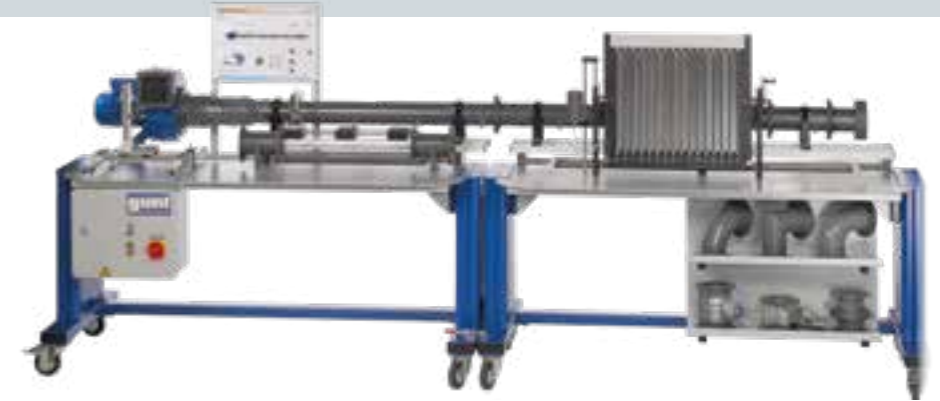
HM 220.02 Measurement of boundary layers Velocity distribution and boundary layer thickness within the boundary layer of a flat plate in longitudinal flow; vertically sliding Pitot tube
