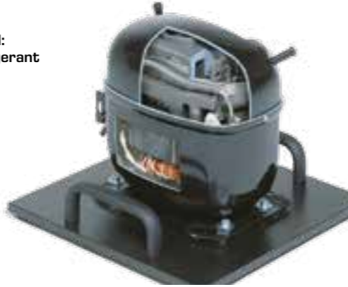
ET 499.03 Cutaway model: open refrigerant compressor, two-cylinder
