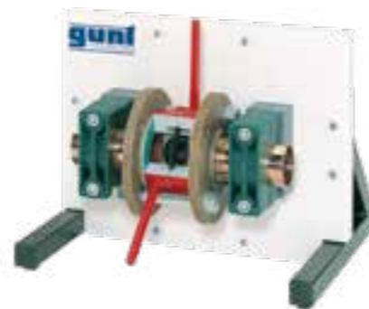
HM 700.02 Cutaway model: flow nozzle
