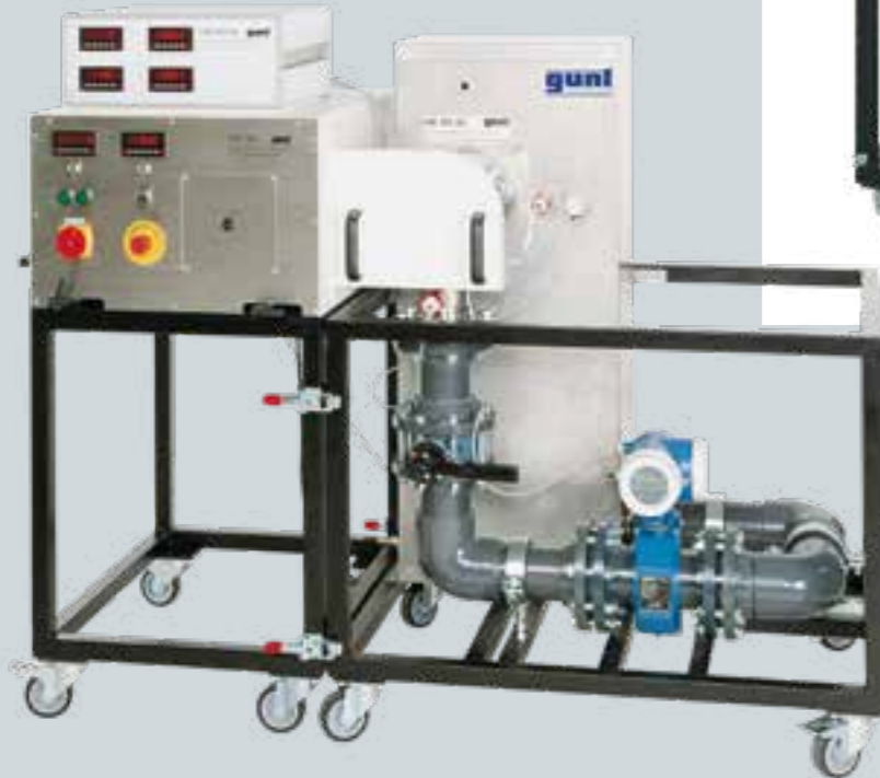
Trainer for an axial pump with axial pump HM 365.45 and drive unit HM 365
