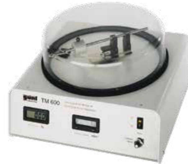
TM 600 Centrifugal force Laws on the behaviour of centrifugal forces on rotating masses
