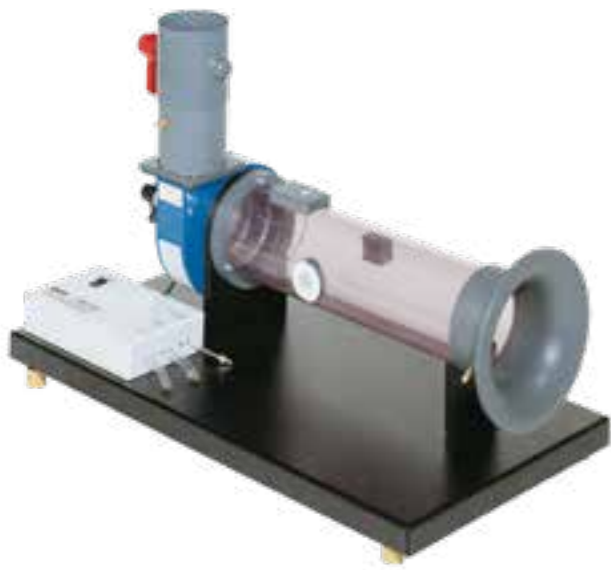
HM 240.05 Pressure losses in pipe elements Measurement of pressure losses in straight pipe sections, in a 90° pipe bend, and in a 90° pipe angle
