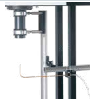
HM 225.07 Free jet Investigation of flow from nozzles
