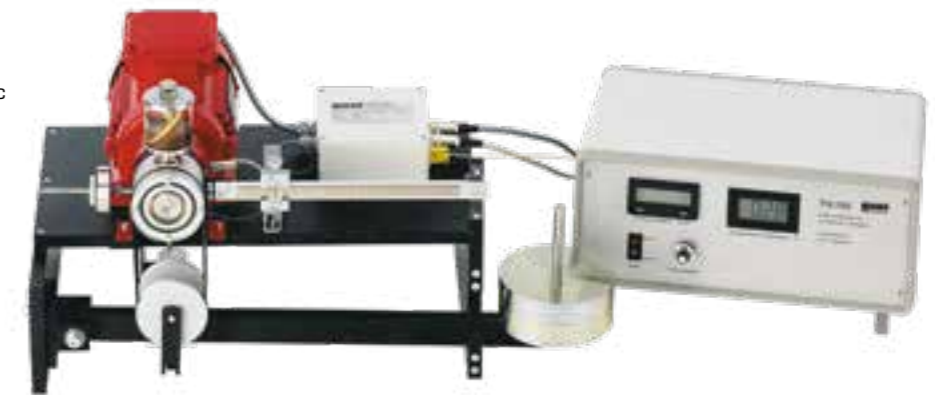
TM 282 Friction in journal bearings Learning the fundamentals of hydrodynamic lubrication by experimentation
