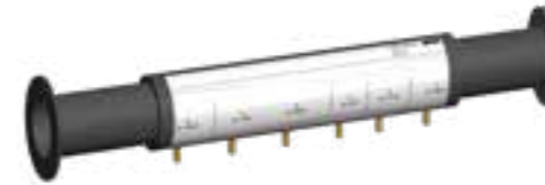
HM 220.01 Venturi tube Examination of the continuity equation and Bernoulli's principle; representation of the pressure curve
