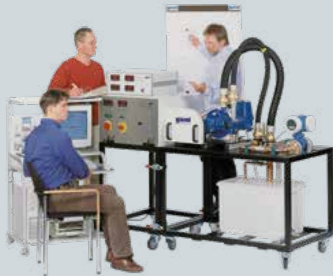
Trainer for positive displacement pumps with supply unit HM 365.10, piston pump HM 365.17 and drive unit HM 365
