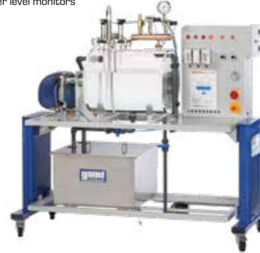
ET 860 Safety devices on steam boilers Familiarisation with boiler safety devices such as pressure and water level monitors
