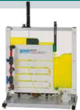
HM 241 Fundamentals of water flow Experiments on water flow in open flumes and in pipes. Transparent design allows observation of the flow processes.
